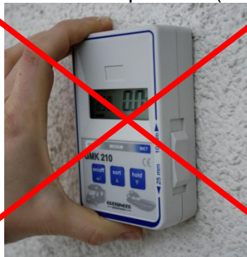
False: unsteady surface
