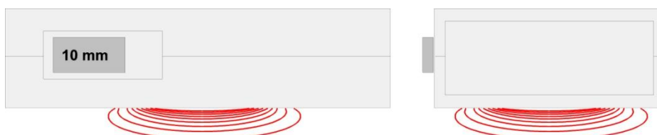
Side view: measuring field and penetration depth for switch setting "10 mm"
