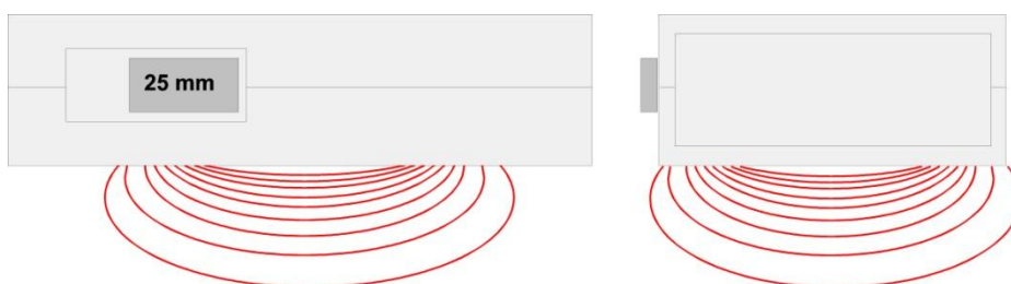
Side view: measuring field and penetration depth for switch setting "25 mm"
