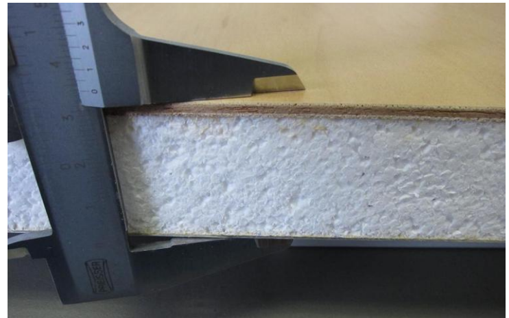
Example sandwich: aluminum - insulation - plywood
