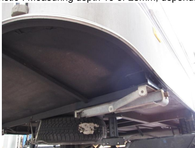
Caravan floor: massive flake board, little protected
