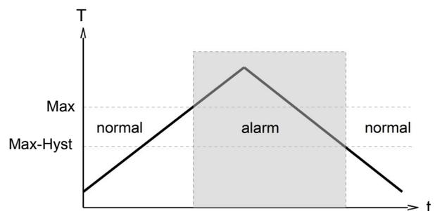
A changeover delay time ( $t_{DS}$ ) can be applied to the switch in the alarm state. Equally, one switch-back delay time ( $t_{DR}$ ) of several can be applied to switching back to the normal state.
