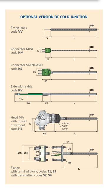
diameter flange with option to mount ceramic terminal block or transmitter (exchangeable measuring insert). Sheath resistance and thermocouple sensors with mineral isolation may be freely bent (resistance sensors cannot be bent in length 40 mm from measuring end) while observing the minimal radius of the bend (5× outer diameter of the sheath).
